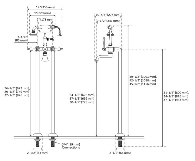
$\label{thm:condition} Underfloor\ access is\ required\ for\ proper\ installation.$  Installation on a concrete slab will require cutting and concrete removal.
