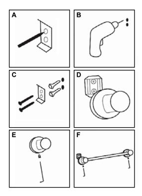
Note: Mount directly to the wall if no mounting bracket is included.
