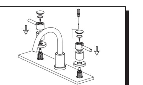
5. Screw escutcheon onto valve body until it is flush with the deck. Install handle, and tighten screw to valve stem.
