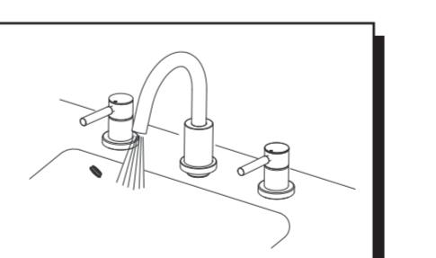
8. After installing faucet, remove Flow Straightener and turn on water to remove any left of debris. Re-assemble Flow Straightener.
