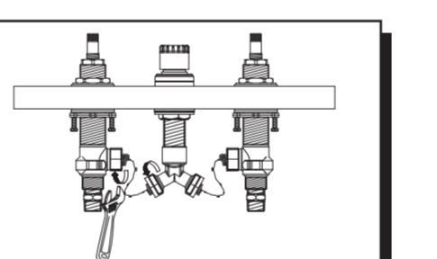
7. Apply pipe tape onto threads of the water supply. Tighten the hose onto water supply.
