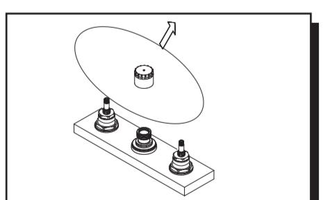
3. Remove the cap and plug from spout tube assembly.
