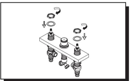
1. Apply pipe tape to spout tube threads and insert spout tube through center hole. From underneath the bathtub, tighten with rubber washer and brass lock nut. Then screw connector onto spout tube.
