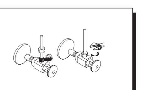
6. Connect handle body and faucet body with water supply tube and tighten with lock nut.
