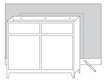
2. Locate and mark the location of the studs to which you will fasten your vanity. You can locate studs by using a stud finder.
