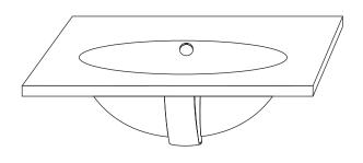
6. At each of the bolt holes in the counter top, attach sink clips by placing the long end of the bracket flat against the sink lip. Screw the wing bolts through the brackets and bolt holes and tighten.
