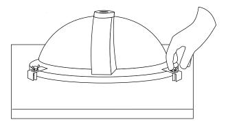
8. Wipe away any excess sealant with a damp cloth, and allow the sealant to dry. Once the sealant is dry, proceed to Step 3.
