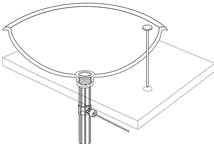
7. Use the link to attach the faucet's lift rod to the drain lever. Pinch the metal clip located on the drain lever to remove. Slide one end of the clip back onto the lever, followed by the link, then the second end of the clip to secure.
