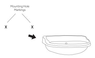
3. Drill pilot holes at the marked locations of the sink's mounting holes. If using anchors, insert the anchors into the drilled holes.
