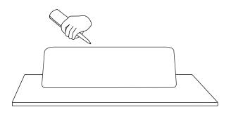
2. Turn the sink right-side-up and position over the drain hole. Set the sink in place, and press firmly to secure.
