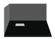
Note: Be sure to leave room for final thinset and tile application. The top of the drain should be level and 1/16" below the adjacent tile.
