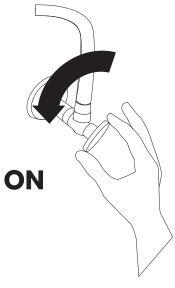
8. Proceed to drain installation. Once complete, turn the faucet on. Check for leaks. Check to ensure that both hot and cold water are running properly. Allow the water to flow for approximately 60 seconds.
