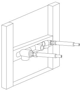
3. Thread the spout's supply tube into the center valve outlet. Tighten firmly using an adjustable wrench. Apply plumber's tape or thread sealant to the threads before attaching.
