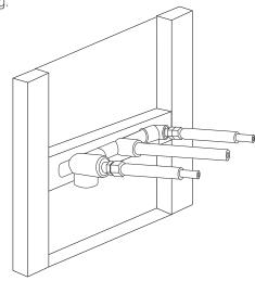
4. Connect the water lines to the faucet body. Use plumber's tape or thread sealant to ensure a watertight connection. If soldering copper pipe, consult a professional.
