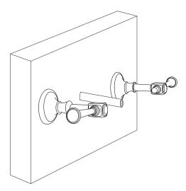
7. Attach the spout by sliding it onto the installed supply tube. Once in place, tighten the set screw on the bottom of the spout using the provided hex wrench.
