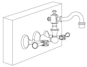
8. Proceed to drain installation. Once installation of the drain is complete, turn on the main water supply. Turn the water on to allow any dust or loose sediment to clear the system. Allow the water to flow through the spout for approximately 60 seconds. Check for leaks. Reattach the aerator once testing is complete.
