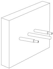
6. Once your finished wall has been completed, attach the faucet handles to the installed stems. Slide the handle onto its corresponding stem, then thread the base onto the stem until hand-tight.
