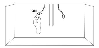
7. Proceed to the drain installation. Once completed, remove the aerator from the spout and turn the faucet on for approximately 60 seconds to remove any dust or loose sediment from the water lines. Ensure that there are no leaks, and that both hot and cold water are running properly. Turn the water off and reattach the aerator.
