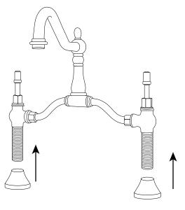
3. From beneath the sink, slide the rubber washers onto the faucet body. Thread the locknuts onto the threaded shanks until hand tight. Tighten firmly.
