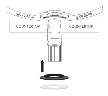
6. Thread the lock nut onto the drain flange. Hand tighten until secure, then finish tightening with a basin wrench once the drain is properly aligned.
