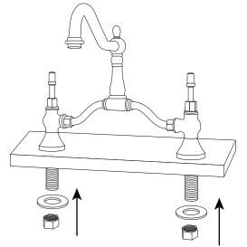
4. Attach the handles to the faucet's valve stems, as shown.
