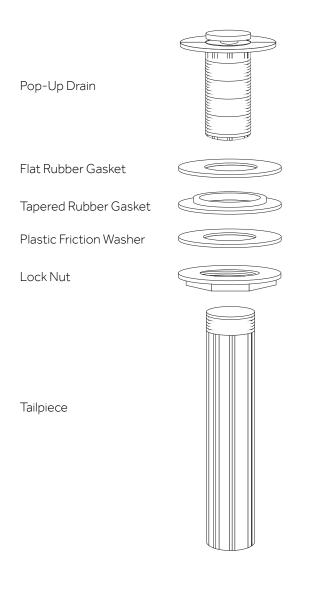
2. Apply plumber's tape to the threading on the tailpiece, then reattach the tail piece to the pop-up drain flange.
