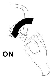
9. Remove the spray nozzle from the faucet, and turn the faucet on for approximately 60 seconds to remove any dust or loose sediment within the water lines. Check for any leaks. Ensure that both hot and cold water are functioning properly. Reattach the spray nozzle once testing is complete.
