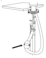
8. Once installation is complete, turn the main water supply back on from underneath your sink. Check for any leaks underneath.
