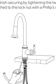
5. Attach the main supply lines to the main water supply. Apply plumber's tape or thread sealant to the threads before tightening. Be very careful not to overtighten.
