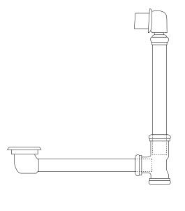
8. Remove the drain and overflow assembly from the tub, and trim the pipes at the marked locations with a hacksaw. Make sure that the blade is suitable for cutting metal
