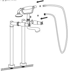
6. When the faucet is installed turn on the water supply, check to make sure that all connections are tight (no water should be leaking) and that the hot and cold supplies are working correctly. Divert the water to the hand shower and allow the water to flow through the hose for approximately 60 seconds.
