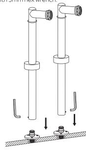
4. Place rubber sealing gaskets in the base of the faucet body and attach to the riser pipes.
