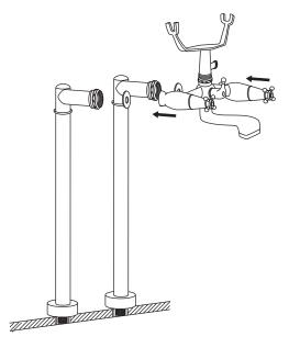
5. Finish your installation by attaching the hand shower hose and handle with the included rubber sealing gaskets.
