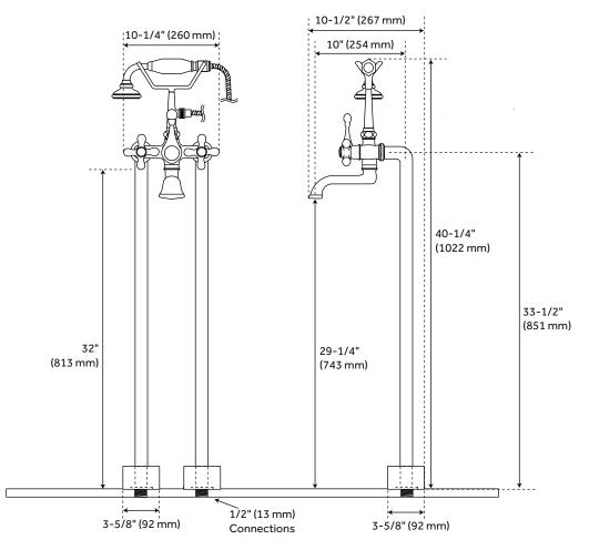
Underfloor access is required for proper installation. Installation on a concrete slab will require cutting and concrete removal.
