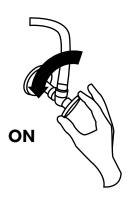
8. Turn the faucet on and ensure that there are no leaks. Check to ensure that both hot and cold water are running properly. Turn on the hand sprayer function and allow the sprayer to run for another 60 seconds, and check for any leaks.
