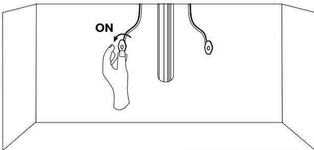
7. Proceed to the drain installation. Once completed, remove the aerator from the spout and turn the faucet on for approximately 60 seconds to remove any dust or loose sediment from the water lines. Ensure that there are no leaks, and that both hot and cold water are running properly. Turn the water off and reattach the aerator.
