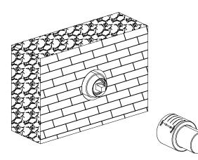
3. When the finished wall is complete, remove the protective cover.
