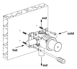
1. Install the valve body. Wrap the threaded portion of the joints in Teflon tape and connect the water inlet and outlet.
