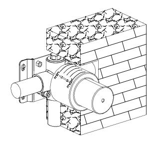
2. Put the protective cover on the valve body and finish the shower wall.
