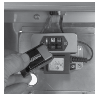
4. Insert and/or replace a new 9V battery
