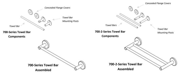
Assemble towel bar by sliding the concealed flange covers over the towel bar mounting posts. Insert the towel bar(s) into the holes on both towel bar posts.
