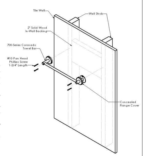
To ensure proper and safe installation, the towel bar should not shift in any direction on the mounting surface.
