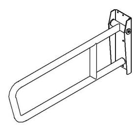
Locate the area with 2" solid wood in-wall backing on the desired mounting surface.
