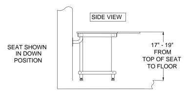
Level the seat by changing the adjustable rubber feet to the desired mounting height (17"-19"). Tighten the lock nuts.
