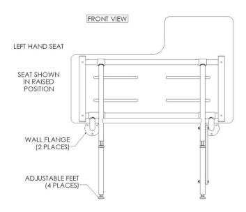
Place the seat in an upright position with the mounting flanges placed firmly against the shower wall.
