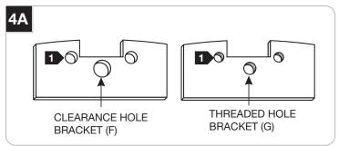
There are four mounting brackets, two with threaded holes and two with clearance holes. Each set uses a clearance hole bracket (F) and threaded bracket (G).
