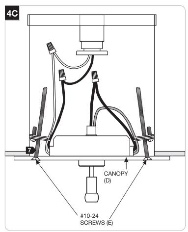
Screw the #10-24 screws (E) through the canopy (D) and into the center hole of brackets until canopy (D) is secured flush to the ceiling.
