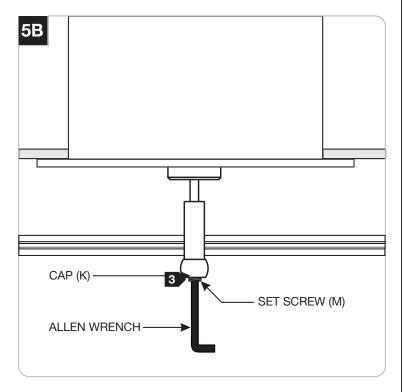
To prevent arcing, tighten the set screw (M) on the bottom of the cap (K) with the supplied Allen wrench.
