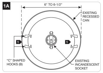
The recessed can transformer can be mounted to down lights that contain: "C" shape hooks (B) on the inside of the can wall, and are 6" to 6-1/2" in diameter.
