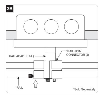
2 Push the rail join connector (J) into the rail adapter (E).
