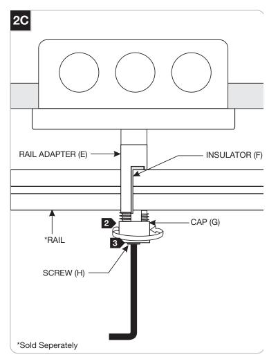
2 Replace and tighten the cap (G) to the rail adapter (E).
