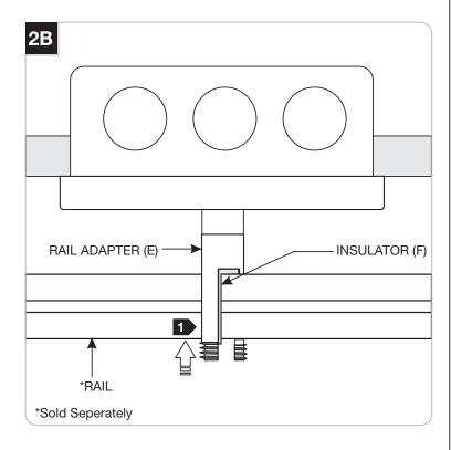
Push the rail into the rail adapter (E) in the middle of insulator(F).
