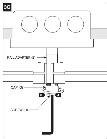
Replace and tighten the cap (G) to the rail adapter (E).
