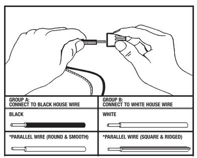
\*Note: When parallel wire (SPT I & SPT II) is used, the tracer wire is square shaped or ridged and less tracer wire is round in shape or smooth. (Seen best when viewed from wire end.) To separate wires, grasp the ends of each wire and pull apart.
