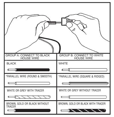
\*Note: When parallel wire is used, the tracer wire is square shaped or ridged and less tracer wire is round in shape or smooth. (Seen best when viewed from wire end.) To separate wires, grasp the ends of each wire and pull apart.
