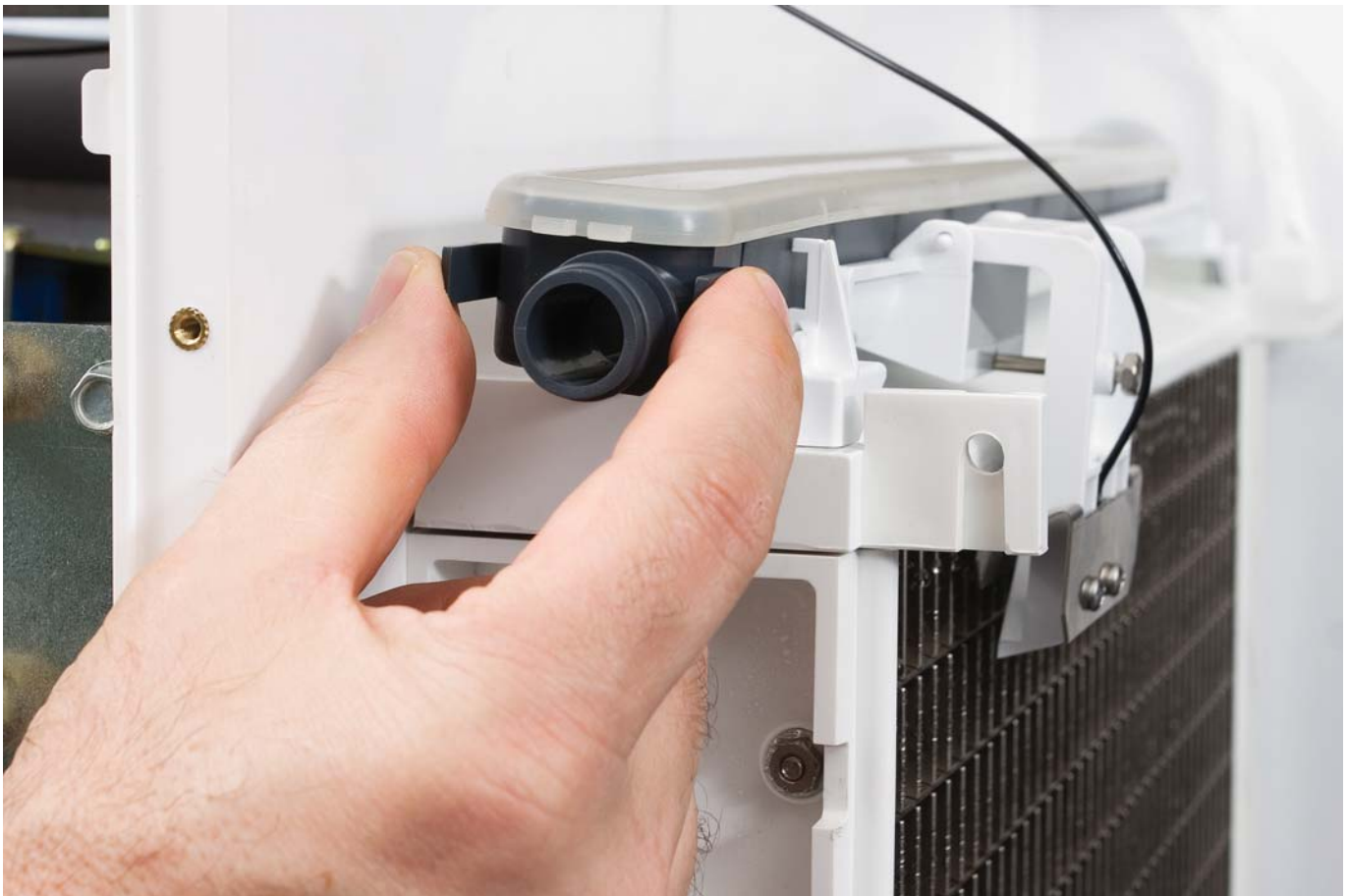
Water Distributor Removal
