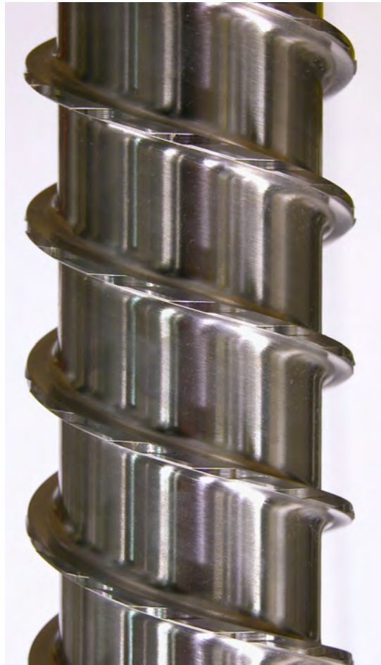
Example of a clean auger
