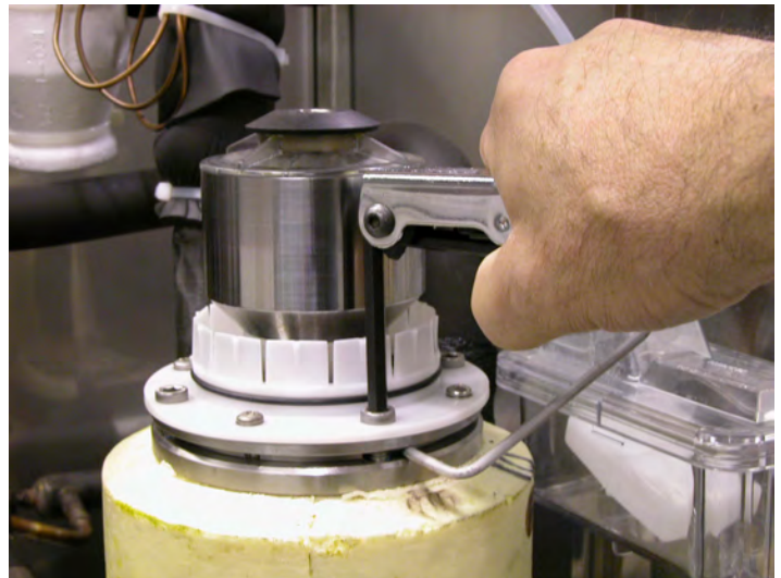
Remove allen head cap screws
