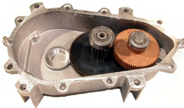
Gear case with First and Second Gears
