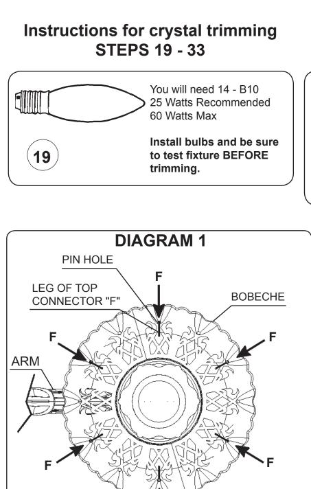
When trimming bobeche with letter "F", insert leg of top connector into pin hole from under bobeche. Hang in every other pin hole starting on either side of the arm (refer to Diagram 1)
