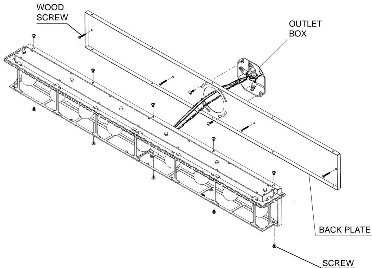
**3** Remove the (10) wall sconce screws and separate the back plate from the wall sconce. Feed stem and ground wires through back plate, then attach to power wires and ground wire in outlet box.
