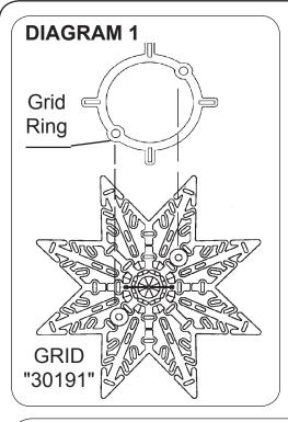
Installation of Grid "30191": Attach (1) Grid "30191" (with finial attached) with two thumb nuts (already screwed onto grid) to 5 ring. Diagram 1. (See page 5 for location on frame)
