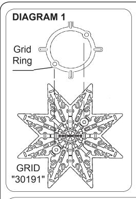
Installation of Grid "30191": Attach (1) Grid "30191" (with finial attached) with two thumb nuts (already screwed onto grid) to 7 ring. Diagram 1. (See page 5 for location on frame)
