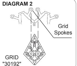
Installation of Grid "30198": Attach (8) Grids "30198" with two thumb nuts per grid (already screwed onto grid) to 4 ring.
