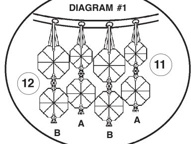
NOTE: SKIP FIRST HOLE AND HOOK CHAINS "A" INTO SECOND HOLE OF RING #1 NEXT TO THE WALL.
