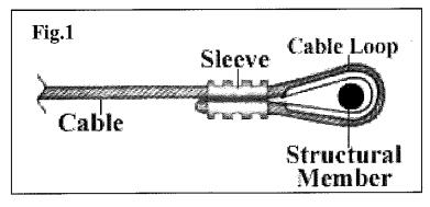
Safety Cable must be mounted on the chandelier **TOP CHAIN LINKS.**
