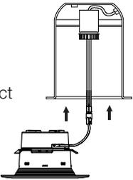
Connect the quick disconnect between the retrofit kit and the medium base umbilical socket.
