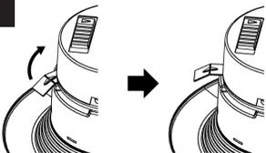
Rotate all three friction clips into the install position as shown below. The clips should be in contact with the locating detent.
