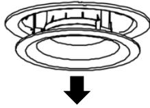
Guide the trim down out of the housing to access the Wattage and CCT selection switch or to disconnect for replacement.
