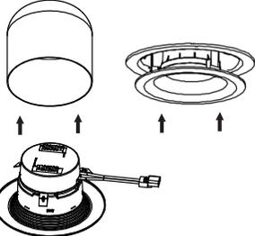
Slide the LED downlight straight up into the recessed housing until the trim is flush with the ceiling. Do not turn the trim counter clockwise or tabs will retract.
