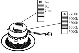
Before installation, select your preferred CCT and Wattage settings by adjusting the sliding switches.
