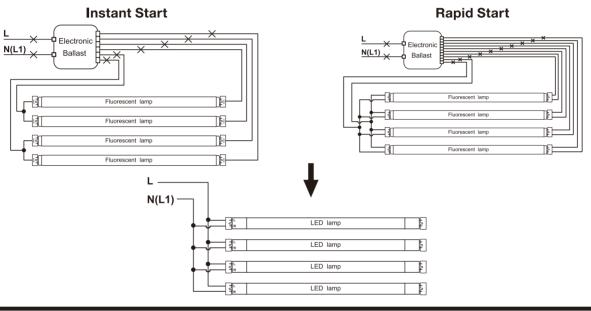
The below ballast wiring represents typical configuration. The actual ballast wiring varies according to ballast model. It is not needed to change socket (if in good condition) to operate double ended lamps, regardless the type of sockets. Make sure one side of fixture is connected to the Live (L) and the other side to Neutral (N).
