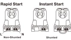
The below ballast wiring represents typical configuration. The actual ballast wiring varies according to ballast model. The socket should be non-shunted.
