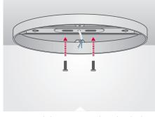
STEP 4: Attach the Mountng Bracket to junction box using 2 screws (provided). Feed all three wires (Postive, negative and ground) from ceiling through center hole of the Mountng Bracket.
