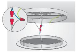
STEP 7: 1. Connect live supply wire (a) (typically black or the smooth, unmarkedside of the two-conductor cord) to live fixture lead (b) with appropriately sized twist on connector.
