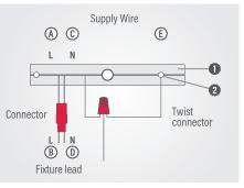
**2.** Connect neutral supply wire © (typically white or the ribbed, markedside of the two-conductor cord) to neutral fixture lead ©.
