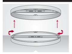
STEP 1: Twist & Unlock Mountng Bracket from lamp unit to remove.
