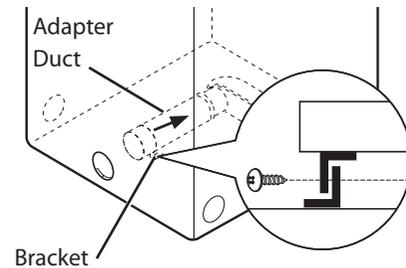
3. Insert the 4-inch (10.2 cm) elbow through the rear opening and press it onto the adapter duct. Be sure that the male end of the elbow faces down through the hole in the bottom of the dryer. Secure in place with duct tape. Attach the cover plate to the back of the dryer with the included screw.
