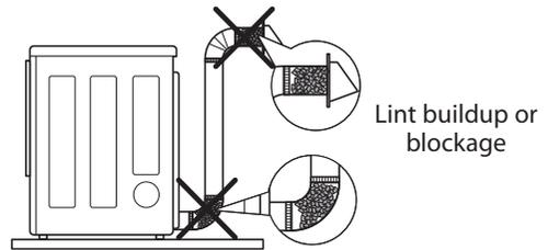
Make sure the ductwork is not crushed or restricted.
