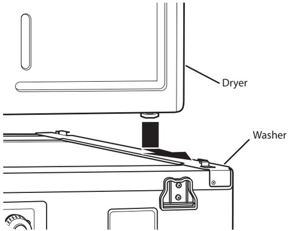
4. Insert the front rail between the bottom of the dryer and the top of the washer. Push the front rail toward the back of the washer until it comes into contact with the side rail stoppers. Install the two remaining screws to secure the front rail to the side rails.
