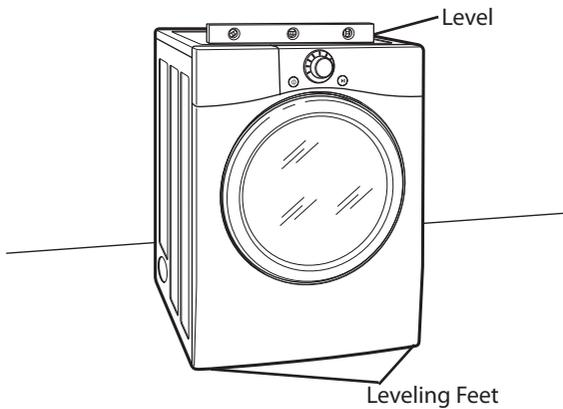
2. Use an adjustable wrench to turn the leveling feet. Turn clockwise to raise the dryer or counterclockwise to lower it. Raise or lower the leveling feet until dryer is level from side to side and front to back.
