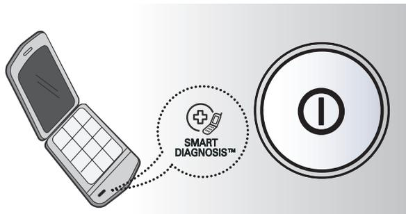
3. Press and hold the Temp Control button for three seconds, while holding the phone mouthpiece to the Smart Diagnosis™ icon or POWER button.
