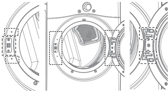
3. Remove the two decorative screws on the left using a screwdriver.
