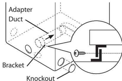
3. Preassemble a 4-inch (10.2 cm) elbow to the next 4-inch (10.2 cm) duct section, and secure all joints with duct tape. Be sure that the male end of the elbow faces AWAY from the dryer. Insert the elbow/duct assembly through the side opening and press it onto the adapter duct. Secure in place with duct tape. Be sure that the male end of the duct protrudes 1½ inches (3.8 cm) to connect the remaining ductwork. Attach cover plate to the back of the dryer with included screw.
