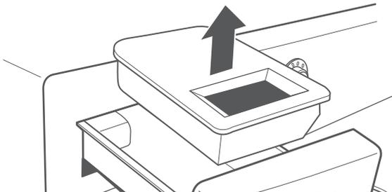
3. Fill the steam feeder just to the filter screen.
