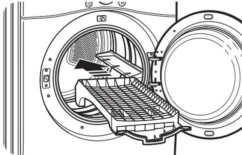
2. Make sure it is seated evenly on the edge of the inner door rim and resting flat on the inside of the dryer.
