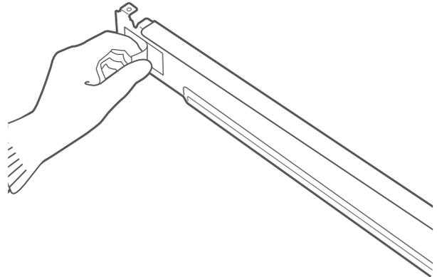
2. Fit the side bracket to the side of the washer top as shown in the illustration below. Firmly press the adhesive area of the bracket to the washer surface. Secure the side bracket to the washer with a screw on the back side of the bracket. Repeat steps 1 and 2 to attach the other side bracket.
