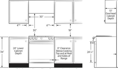
\*Side clearance above cooking surface to any objects, i.e., wall.
