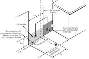
Recommended area for gas piping and electrical outlets. Recommended area for 100% electrical outlet (air fryer).
