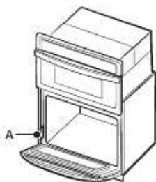
Combi oven A. Model/serial/rating plate
