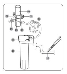
01 Cold water line 02 Pipe clamp 03 Plastic line 04 Compression nut 05 Compression sleeve 06 Packing nut 07 Shut off valve 08 Filter cartridge 09 Cartridge holder 10 Cut vertically by 90 degrees
