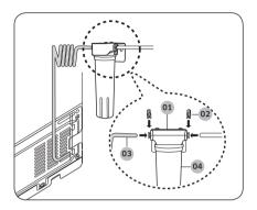
01 Cartridge holder02 Plastic clip03 Plastic line04 Filter cartridge
