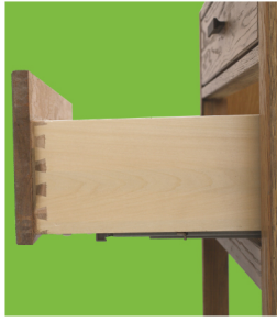
Dovetailed drawer construction
