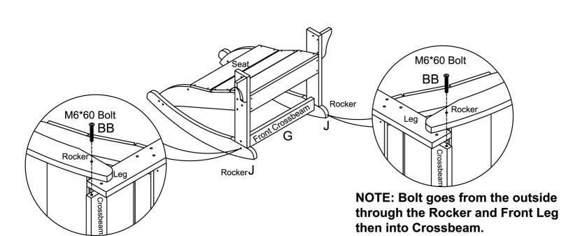
**STEP 3A:** Attach the back of the Rockers (Part J) to the seat (Part B) using (2) M6\*60 Bolt and Nut Sets (Part CC).
