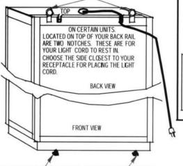
NOTE: USE ADJUSTABLE GLIDES TO LEVEL DOORS AFTER SET-UP. ALIGN SLIDING DOORS BY TURNING GLIDES UP OR DOWN UNTIL DOORS ARE LEVEL AT THE TOP AND BOTTOM. ALSO USE TO LEVEL UNIT ON **UNEVEN FLOORS**
