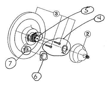
MOUNTING SCREWS+CAM+DIVERTER ASSEMBLY 2303-1210 MOUNTING SCREWS
