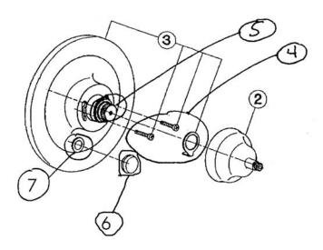
MOUNTING SCREWS+CAM+DIVERTER ASSEMBLY 2303-1210 MOUNTING SCREWS
