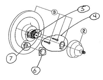
MOUNTING SCREWS+CAM+DIVERTER ASSEMBLY 2303-1210 MOUNTING SCREWS
