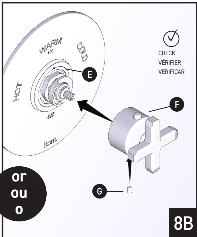
1. Install Handle\* (F) to valve body. Check handle alignment and engagement. Secure with Hex Screw (G). **NOTE:** Adjust the temperature on an open outlet to 100°F. Install the handle with the button at 12 o'clock position.
