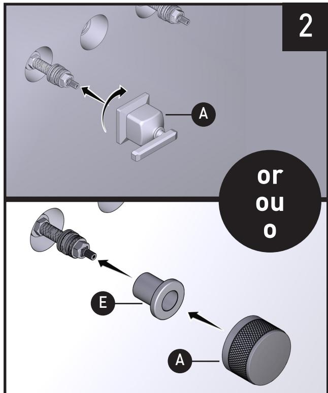
Install Handle (A) onto valve adapter **OR** install valve flange (E) and then install Handle (A) until fully seated.
