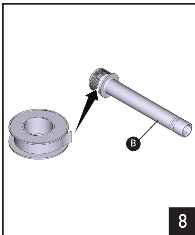
Wrap Thread Seal Tape 3 turns around end of Spout Stem Adapter (B).
