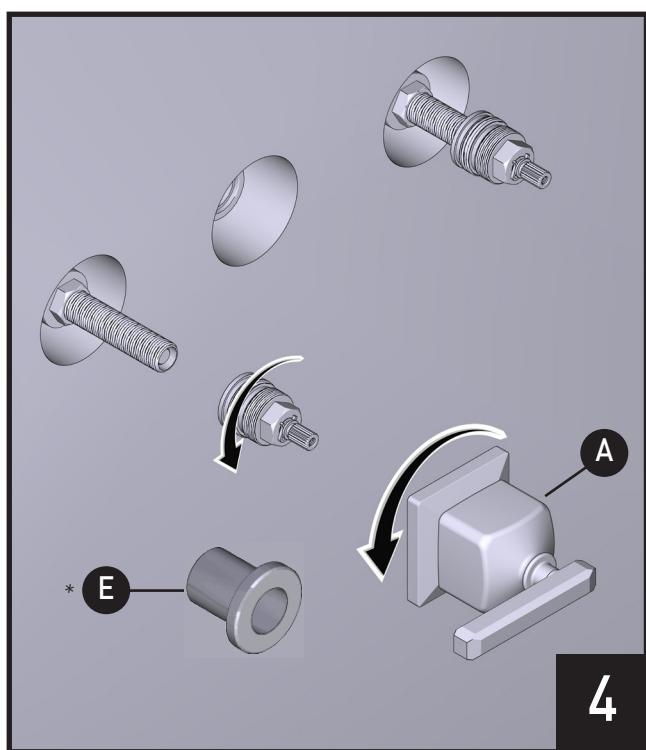
Remove Handle (A) and handle valve adapter (*and Valve Flange (E) if applicable*) from valve threads (x2).
