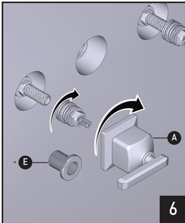
Install Handle (A) and handle valve adapter (*and Valve Flange (E) if applicable*) onto shortened valve threads (x2).
