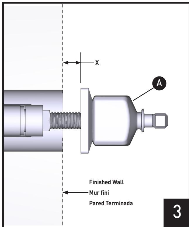
If a gap remains once handle is installed, measure distance from finished wall to handle base.
